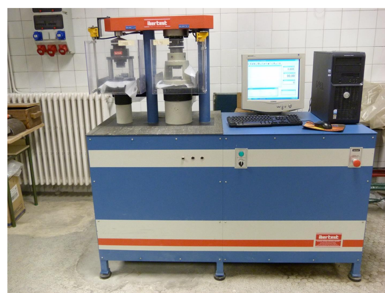
Fig. 2 Machine used for flexural and compressive strength tests.
