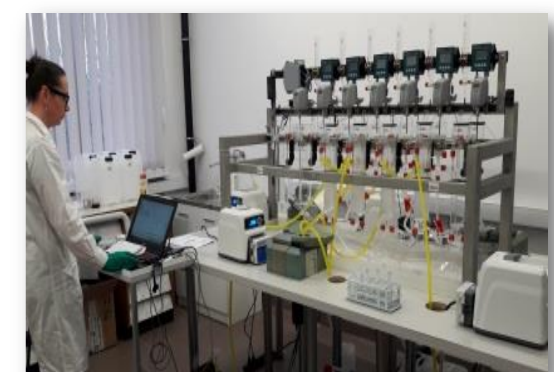
Pilot plant mixer-settlers system for the continuous countercurrent solvent extraction process (SX Kinetics Inc., Canada).
