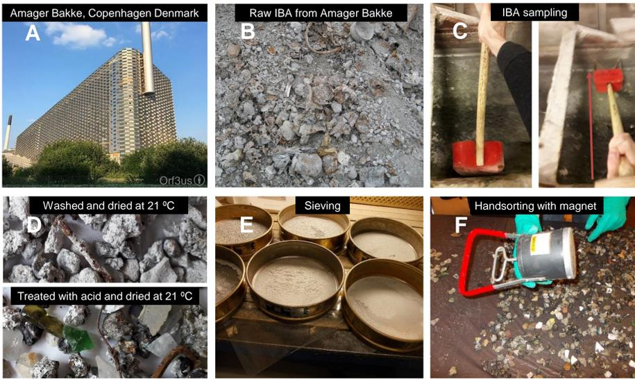
Fig. 1: A. Amager Bakke (WtE plant), B. IBA, C. IBA sampling, D. IBA treated/non-treated, E. Sieving, F. Characterisation.
