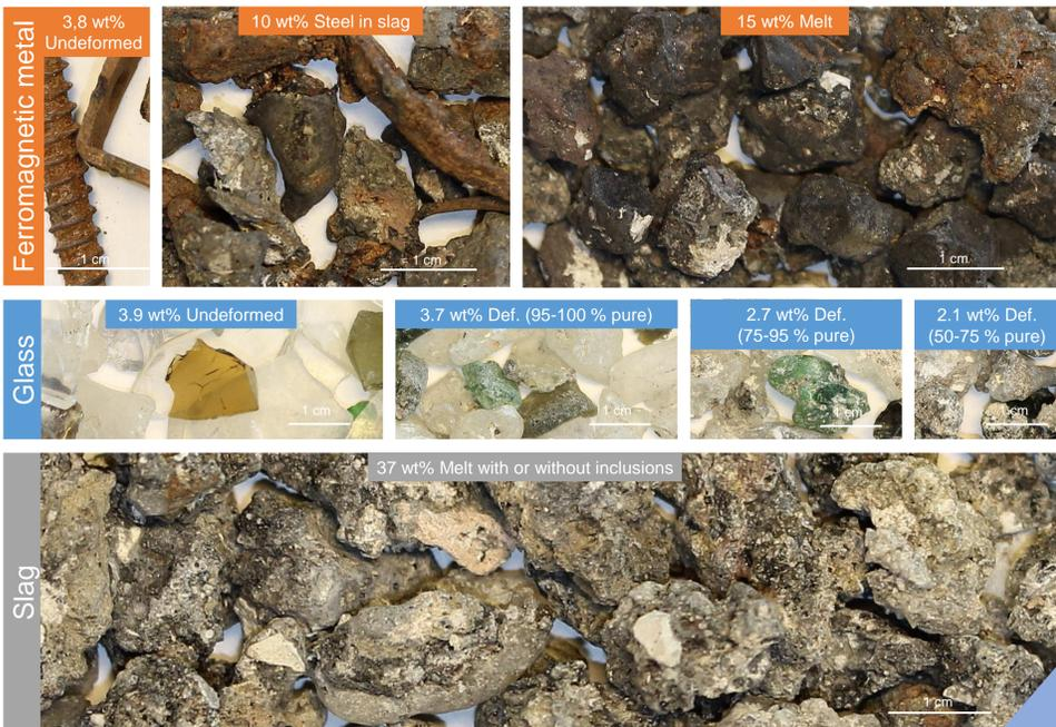
Fig. 3: Diagram with the assorted material categories displaying example photos. Diagram is not showing diamagnetic metal, ceramics and mineral construction material. Percentages refer to composition of 2-63 mm IBA fraction.
