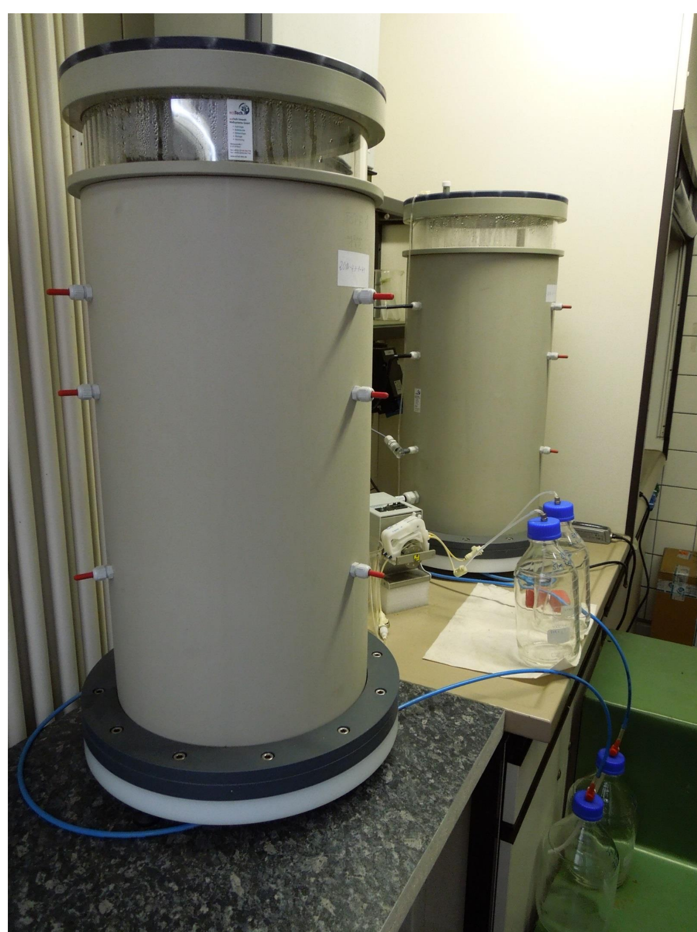
Fig. 1: BAM's lysimeter test rig. The volume of the vessels is 40.6 L.
