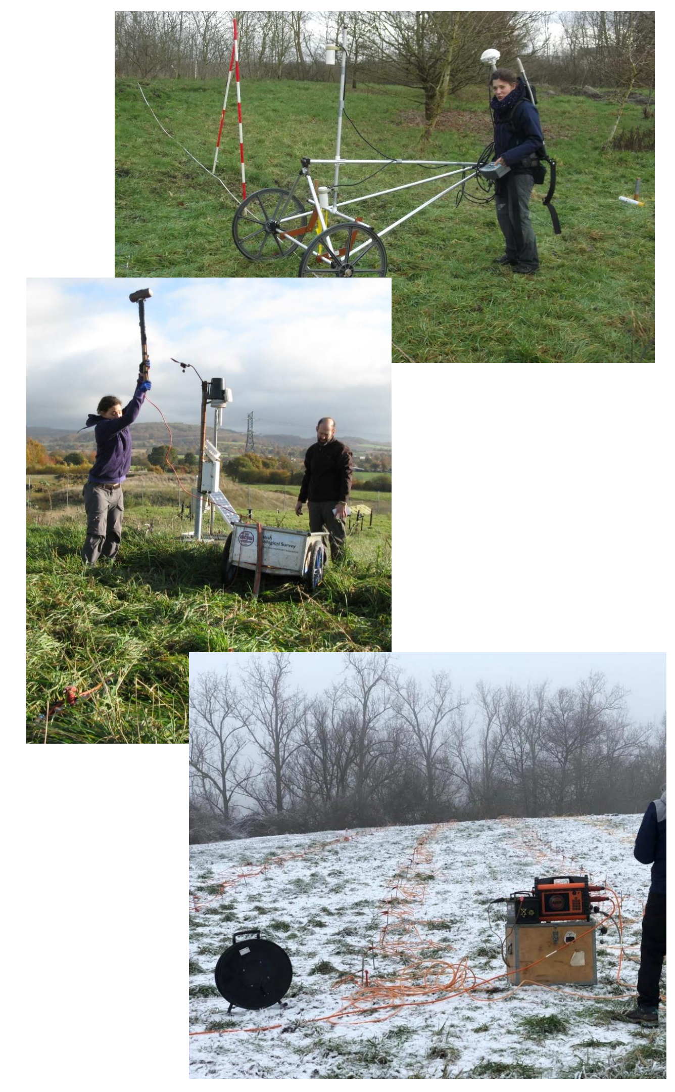
Fig. 4. Magnetometry (top), EMI (middle) and ERT/IP (bottom) acquisition.
