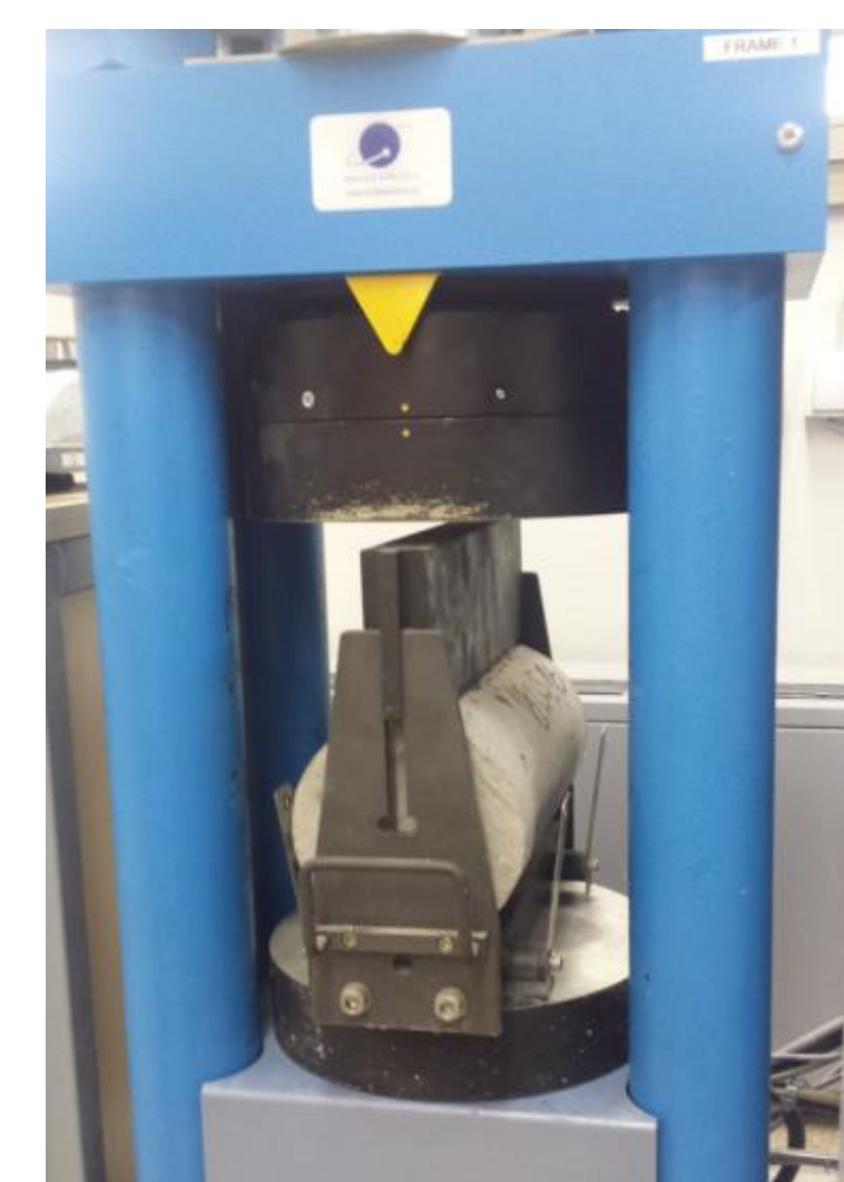
Brazilian method – testing of specimen with splitting test
