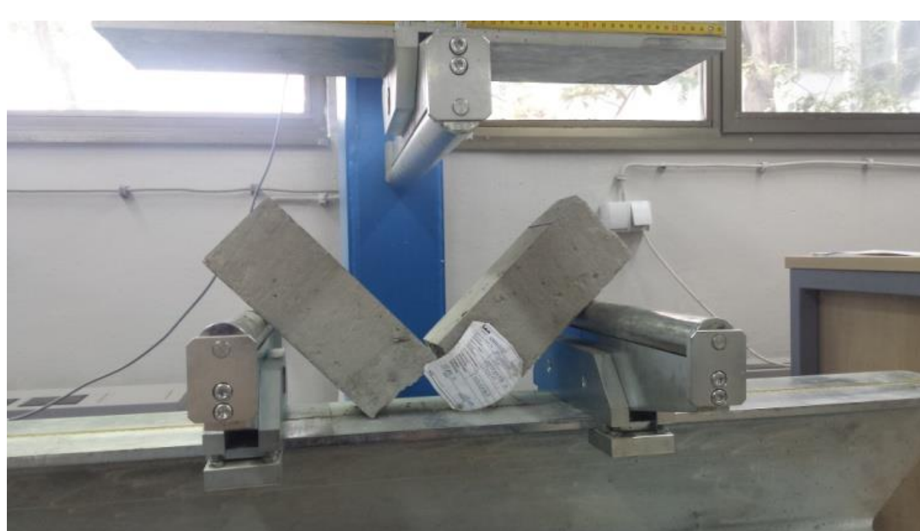
Prisms tested to bending
