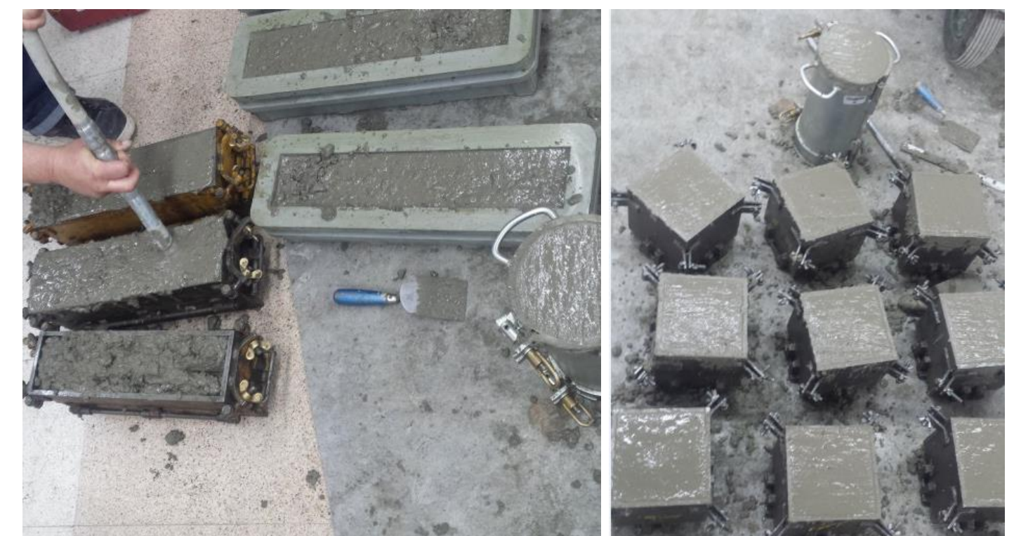
Preparing of concrete samples
